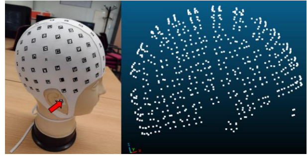
Figure 2: Left: cap used for data capture. Right: 3D point cloud of the head obtained with the PhotoMeDAS app.
